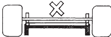
Floor tray. Showing legal and illegal. Illegal is defined as creating a skirt effect.
